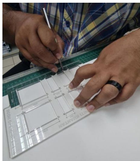
Figure 1 : ARCHICUT template are used to cut model board for door and window openings.
